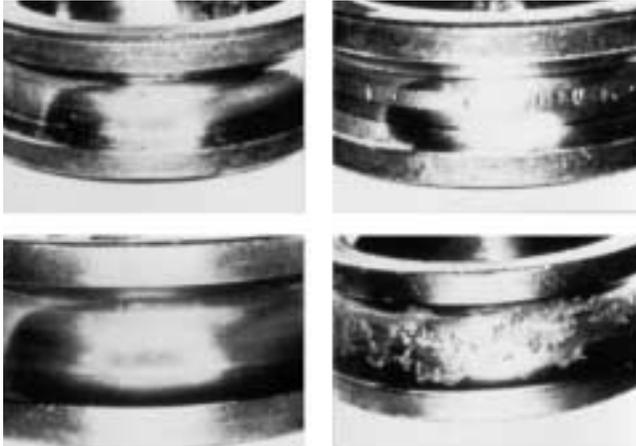
If the bearings continue to operate with inadequate lubrication, the evidence that shows this to be the mode of failure becomes destroyed. Notice how the spherical bearing rollers shown in Figure 9 become damaged with continued operation.
