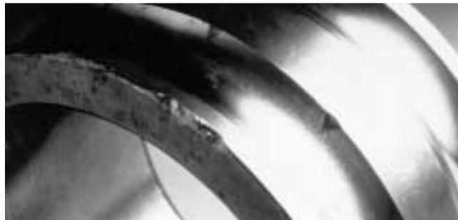
of serious fretting corrosion. Microscopic movement between the shaft and the bore causes the rust colored patches to develop. Small amounts of fretting are common with setscrew mounted bearings and are not detrimental to bearing life. Advanced cases, caused by loose mounting, can lead to cracks.
