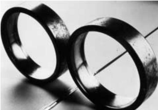
Figure 22. Smearing on a Bearing Race
