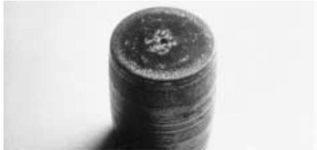
Figure 16. Puddle Corrosion
