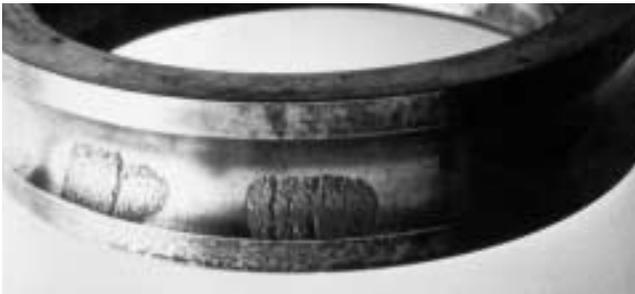
Figure 21. Two Load Zones on the Outer Race
