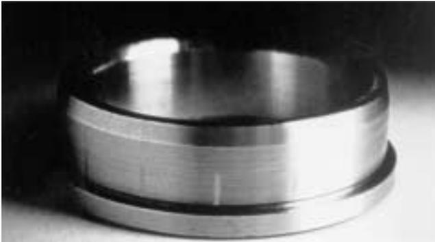
Figure 20. Spalls Resulting from True Brinneling
