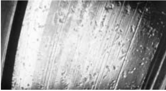
Figure 15 shows a spherical roller bearing roller that has rusty ends from moisture in the lubricant.
